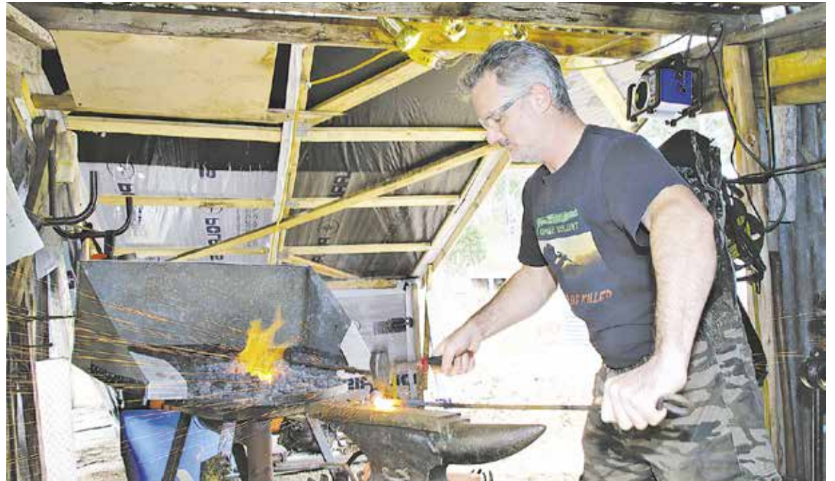
The growling anvil works a piece of recycled metal to make a fire poker. Photo by: Mike Moores
