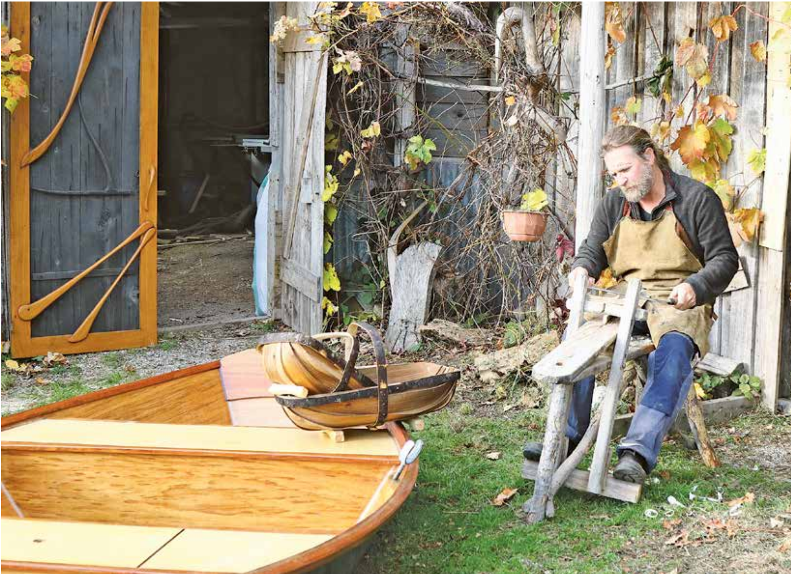
Michael Thomson shapes timber on his 'shave horse' with a 'draw knife' to make a traditional flower basket. Photo by: Mike Moores
