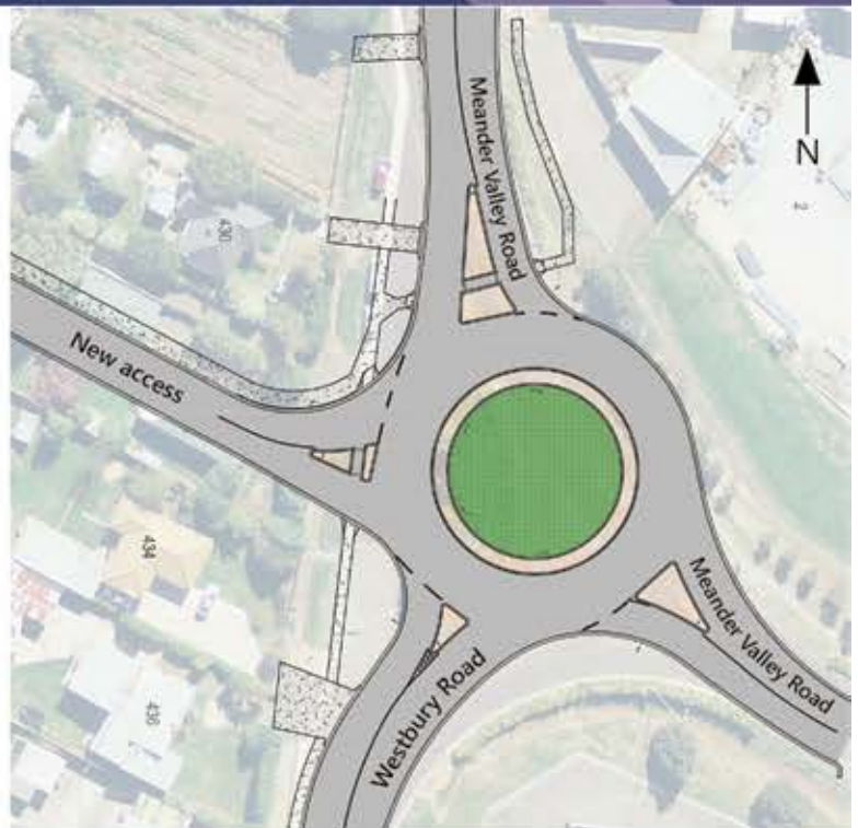
Above: The new roundabout to be constructed at the intersection of Westbury Road and Meander Valley Road in Prospect Vale.
